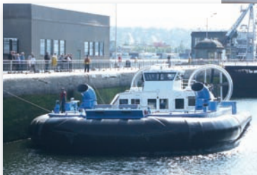
The massive Suna-X hovercraft is 98 feet long and 50 feet wide and can carry 50 passengers and 22 tons of freight. Kvichak Marine Industries.
