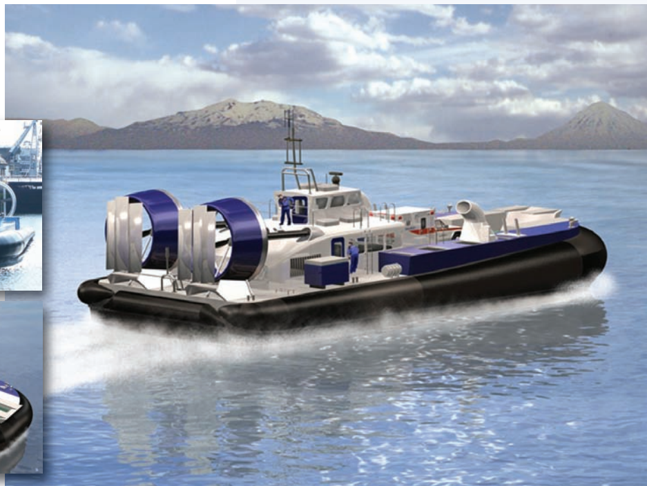
The massive Suna-X hovercraft is 98 feet long and 50 feet wide and can carry 50 passengers and 22 tons of freight. Kvichak Marine Industries.
